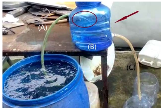
Gambar 6 . Sistem vakum, A= selang hisap, B = container air, C = selang keluar
