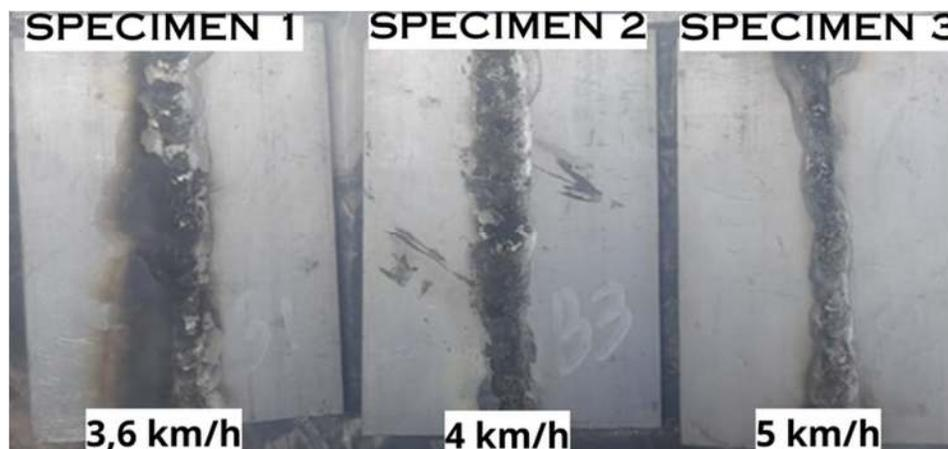
[Figure 2](#). TIG welding results on aluminum 6061
