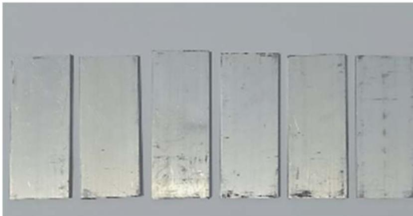
Figure 1. Al6061 plate with dimensions 100x40x4 mm
