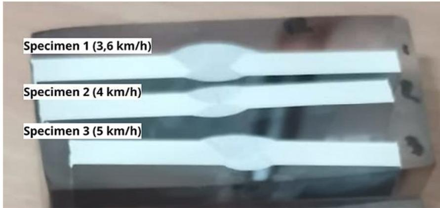
Figure 3. Preparation of vickers hardness testing specimens
