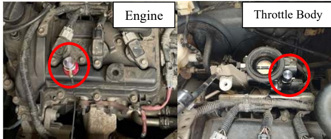
Figure 3. Placement of vibration accelerometer sensors.
