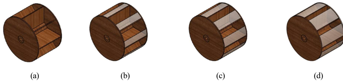
Figure 1. (a) Water wheel without cover, (b) Water wheel with 1/3 cover,(c) Water wheel with 1/2 cover, (d) Water wheel with 2/3 cover.
