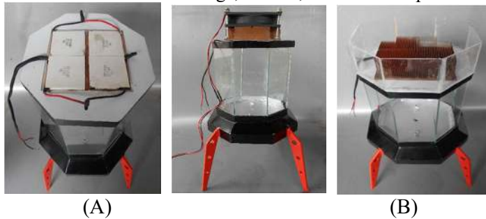
Figure 1. A) Installation of TEG, and B) Installation of cooling system on candle tubes
