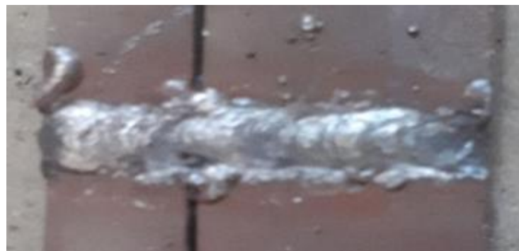
Figure 6. The welding results of 4.5 cm pre-heating distance
