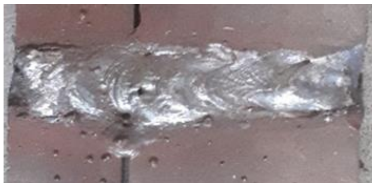
Figure 5. The welding results of 3 cm pre-heating distance
