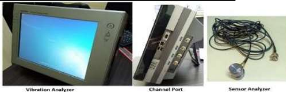
Figure 3. ONO SOKKI FFT ANALYZER and accelerometer sensor.
