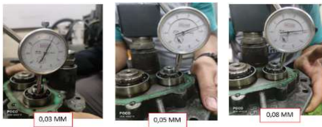
Figure 5 . GAP Clearance distance settings 0.03, 0.05, 0.08 mm
