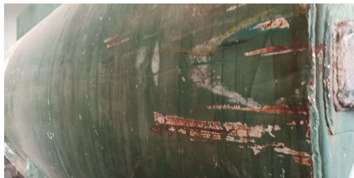
Figure 3. Scratches on the tank's paint covering
