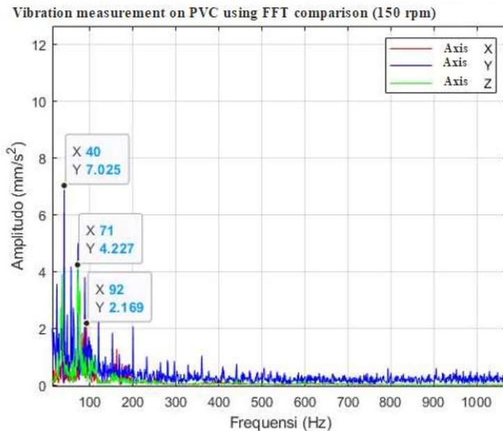
**Figure 14.** FFT outcomes on PVC at 150 rpm rotating speed
