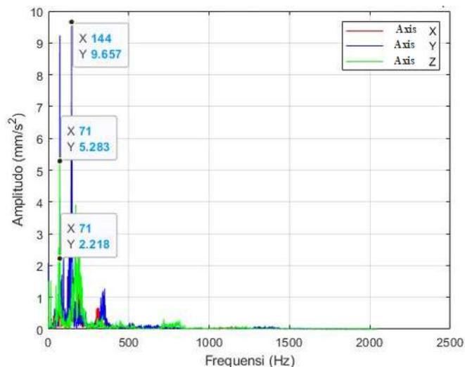
**Figure 12.** Shows the FFT outcomes on aluminum at 150 rpm.
