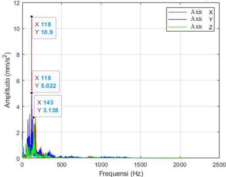
**Figure 15.** FFT outcomes on wood at a 95 rpm rotational speed
