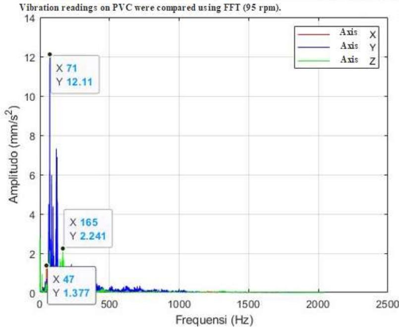
**Figure 13.** Shows the FFT outcomes on PVC at 95 rpm.
