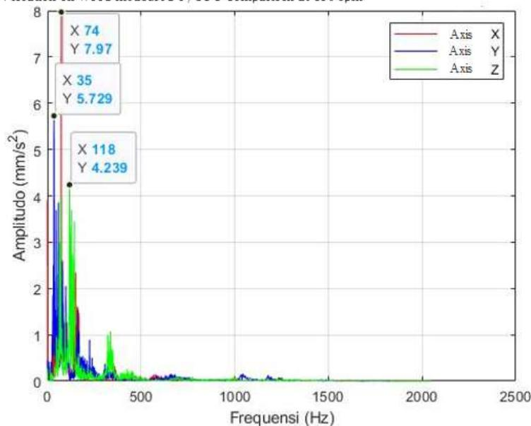
**Figure 16.** Shows the FFT outcomes on wood at 150 rpm.
