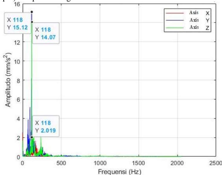
**Figure 11.** Shows the FFT outcomes on aluminum at 95 rpm.
