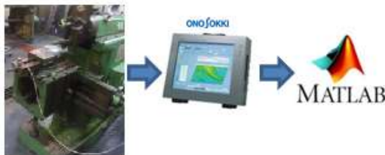
Figure 4. FRF Measurement Test Set Up.
