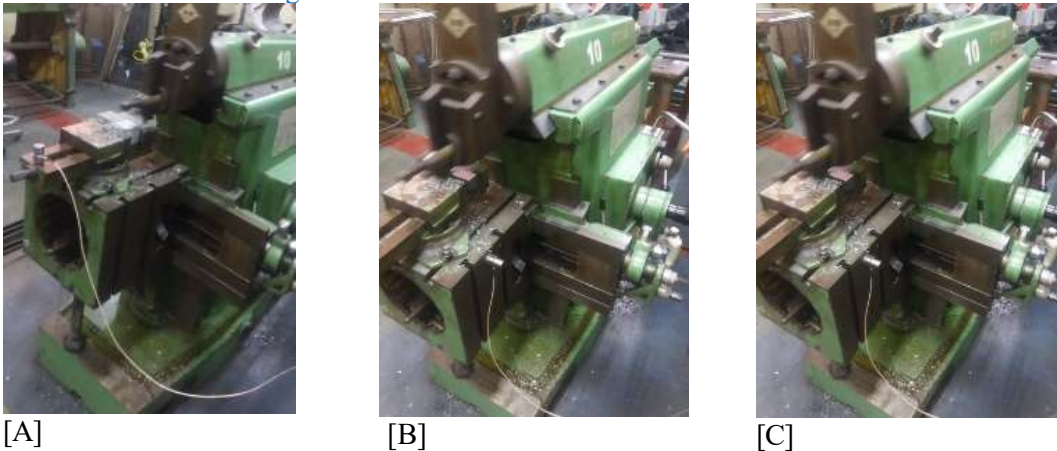
Figure 3. Position of FRF measurements in the direction of [A] X-axis, [B] Y-axis, [C] Z-axis
