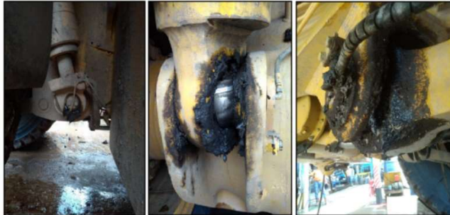
Figure 9. Condition of wet pins and bushings.
