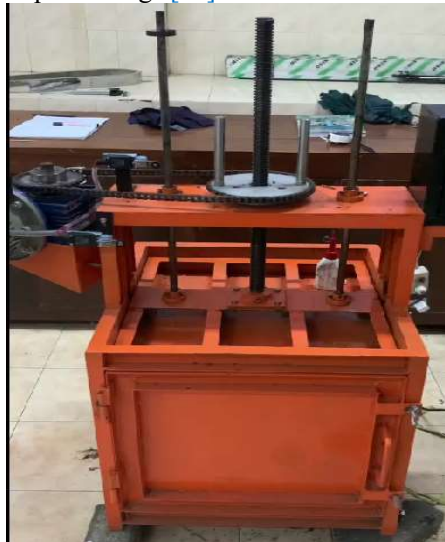
Figure 7. The finished product of a plastic waste press machine using a 1 Hp AC motor.
