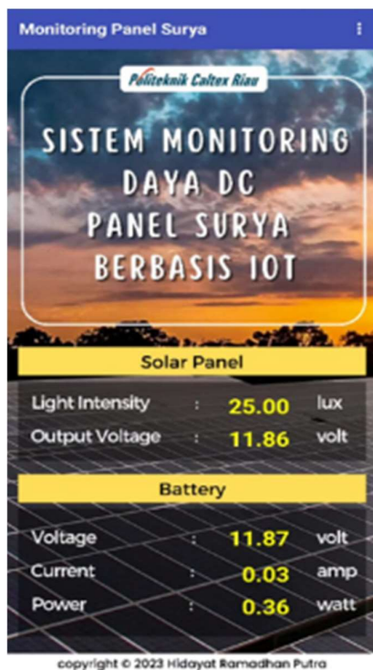
Figure 11. Solar panel monitoring interface application using MIT App Inventor
