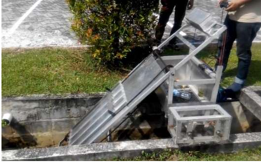
Figure 10. Prototype of machine tool for transporting bottle waste in ditches.
