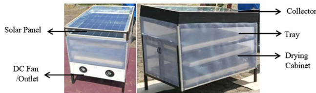
Figure 3. PV/T solar dryer
