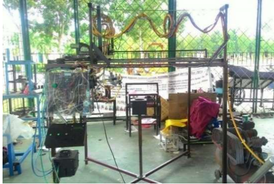
Figure 7. Front view of a painting robot with three-axis movement
