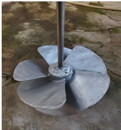
Figure 3. Whirlpool turbine blades.
