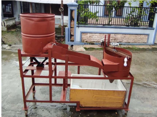
Figure 2. Hydroelectric power plant prototype
