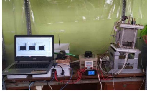
Figure 5. Photograph of pool boiling test facility
