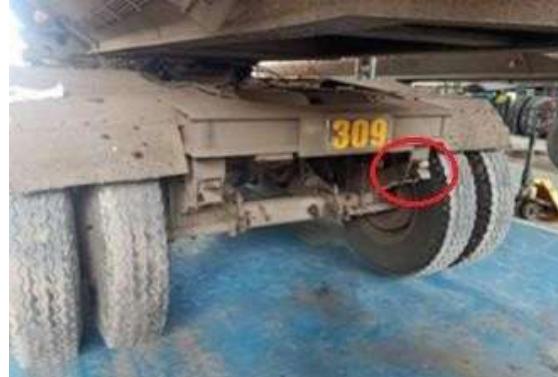
Figure 3. Hanger welding defect
